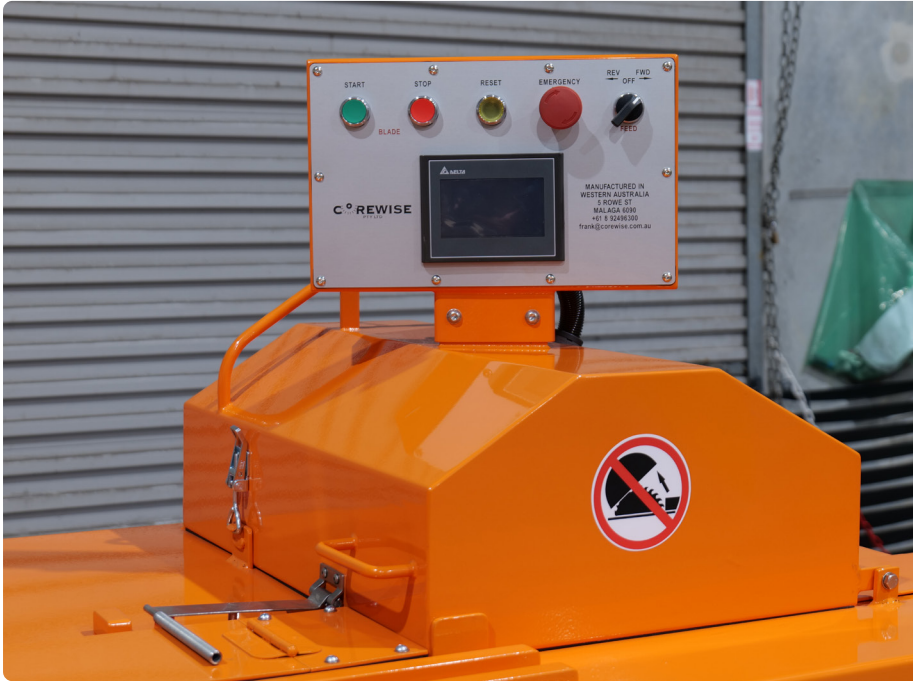
Blade cover housing with lock down latches and water tap
